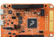
The Freescale Freedom development boards are small, low-power, cost-effective evaluation and development platforms perfect for quick application prototyping and demonstration of Kinetis MCU families and Freescale sensors. These evaluation boards offer an easy-to-use mass-storage device mode flash programmer, a virtual serial port and classic programming and run-control capabilities. Get started at [freescale.com/FRDM-K82F](http://freescale.com/FRDM-K82F).
