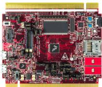
The TWR-K80F150M development board is designed to work in standalone mode or as part of the Freescale Tower System, a modular development board platform that enables rapid prototyping and tool re-use through reconfigurable hardware. Order your Tower System evaluation board today at [freescale.com/TWR-K80F150M](http://freescale.com/TWR-K80F150M).
