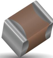
X7T formulations are called "temperature stable" ceramics and fall into EIA Class II materials. Its temperature variation of capacitances within +22%/-33% from -55°C to +125°C. This capacitance change is non-linear. Capacitance for X7T varies under the influence of electrical operating conditions such as voltage and frequency. X7T dielectric chip usage covers the broad spectrum of industrial applications where known changes in capacitance due to applied voltages are acceptable.
