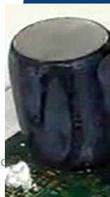
Ballooning sleeve caused by water entrapment during aggressive washing of a large electrolytic
