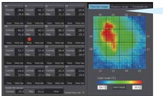
Confirm the temperature status by simultaneously displaying the temperature data and thermal image. Easily identify the device which is outputting an alarm.
