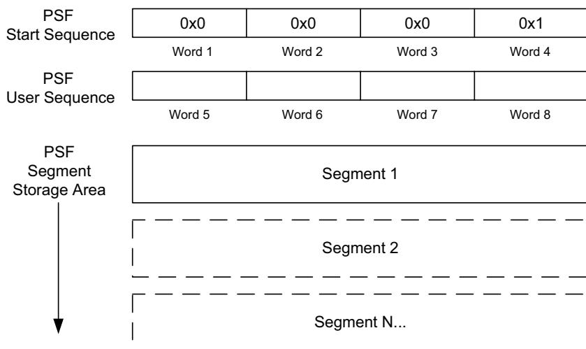
**Figure 6-1: High-Level Format of a PSF (PMD Structured Data Format) Memory Space**
