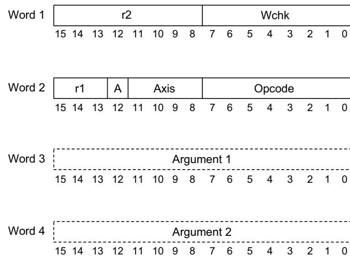
This is shown in [Figure 6-4](#) which shows the overall sequence and format for NVRAM commands. The following table details the content of these words:
