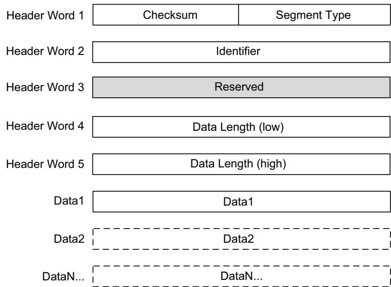
The central mechanism which PSF provides to store data is called a data segment. PSF data segments come with their own headers which allow structuring and data integrity checks of the PSF memory space. [Figure 6-2](#) shows the format of a PSF data segment. The following section details each of the elements in this data structure.
