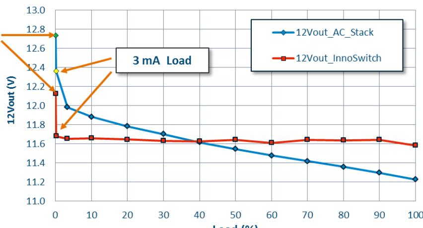
12 V Output regulation (zero load on 5V Main output)
