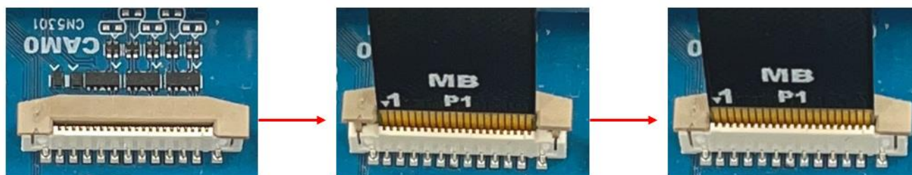
Figure 4-4 Genio 360P/360 (MT8367/MT8366) EVK Camera FPC Installation
