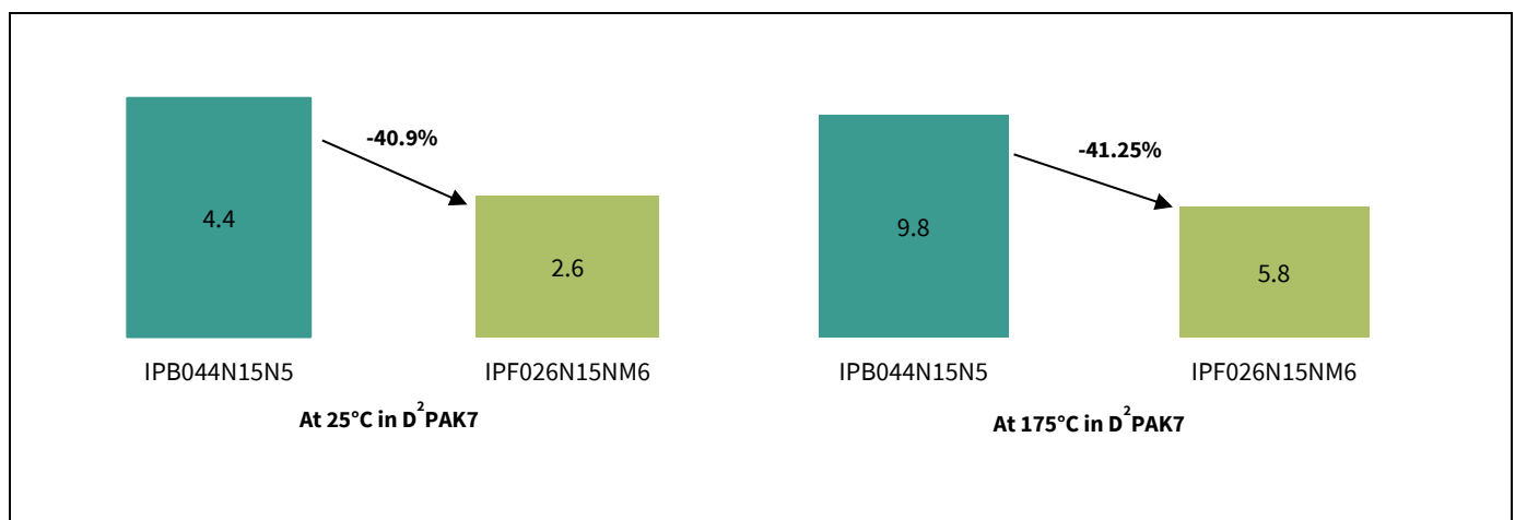
Figure 2 Comparison between the maximum R_{DS(on)} (mΩ) for OptiMOS™ 6 150 V and OptiMOS™ 5 150 V MOSFETs in D²PAK7 for 25°C (left) and for 175°C (right)
