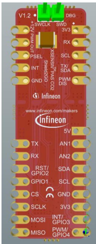
Figure 2 Pinout XENSIV™ PAS CO2 Shield2Go
