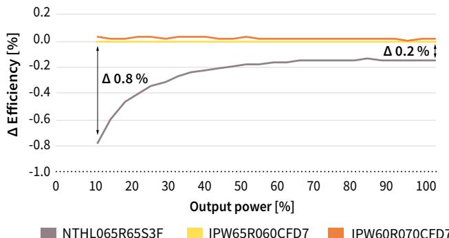
The 650 V CoolMOS™ CFD7 family increases efficiency over the whole load range. Thanks to the improved gate charge ( $Q_g$ ) and the fast switching performance, in light-load conditions 0.8 percent while in full-load conditions 0.2 percent higher efficiency is achievable compared to alternative offerings in the market.
