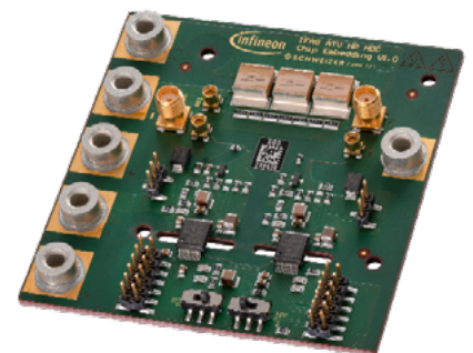
Figure 2: Smart p 2 Pack® demonstrator board with 1200 V CoolSiC and 3rd generation EiceDRIVER™
