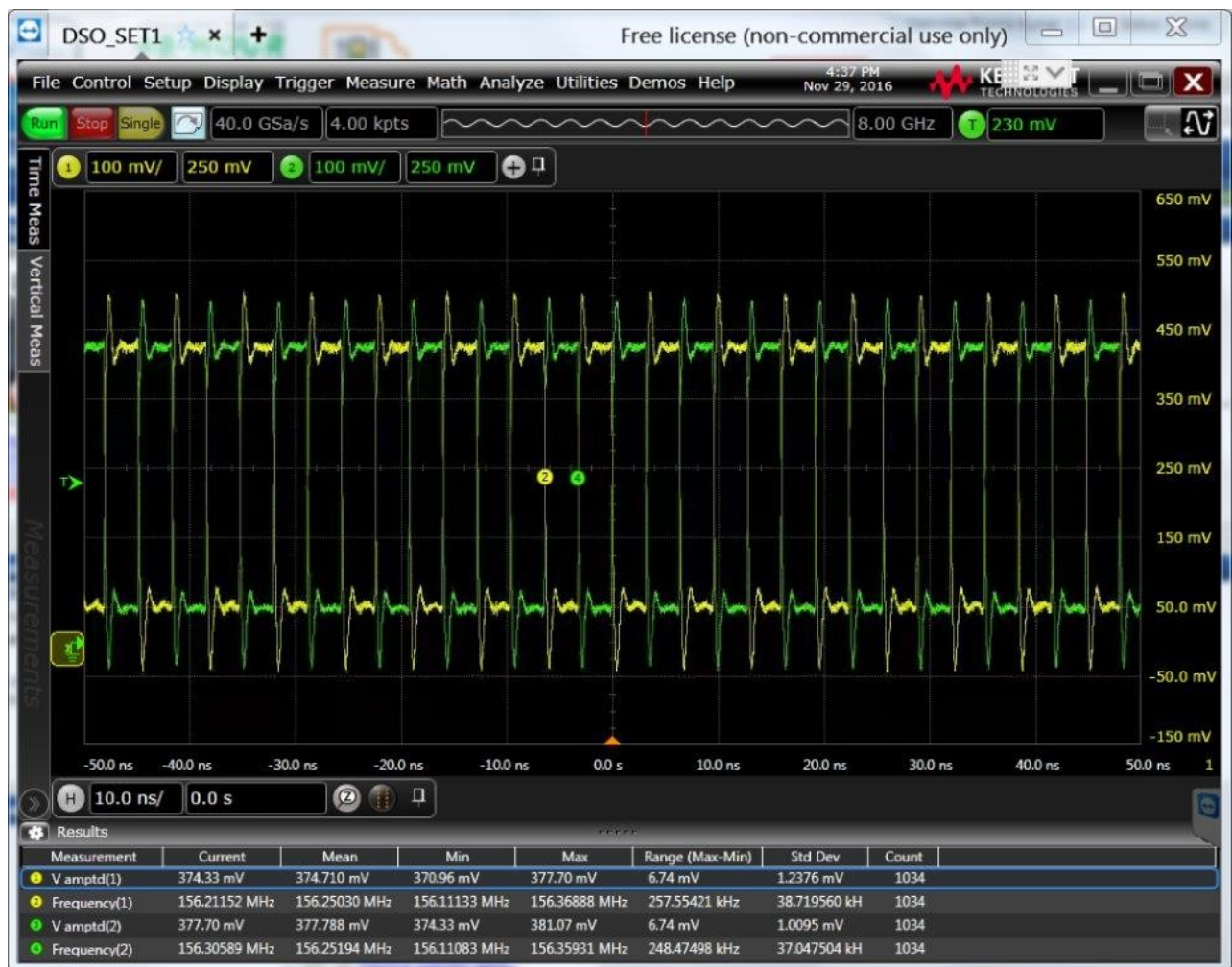
Figure 5-1. CY29412FLXI Differential Output of 156.25 MHz and Output Standard as LVPECL
