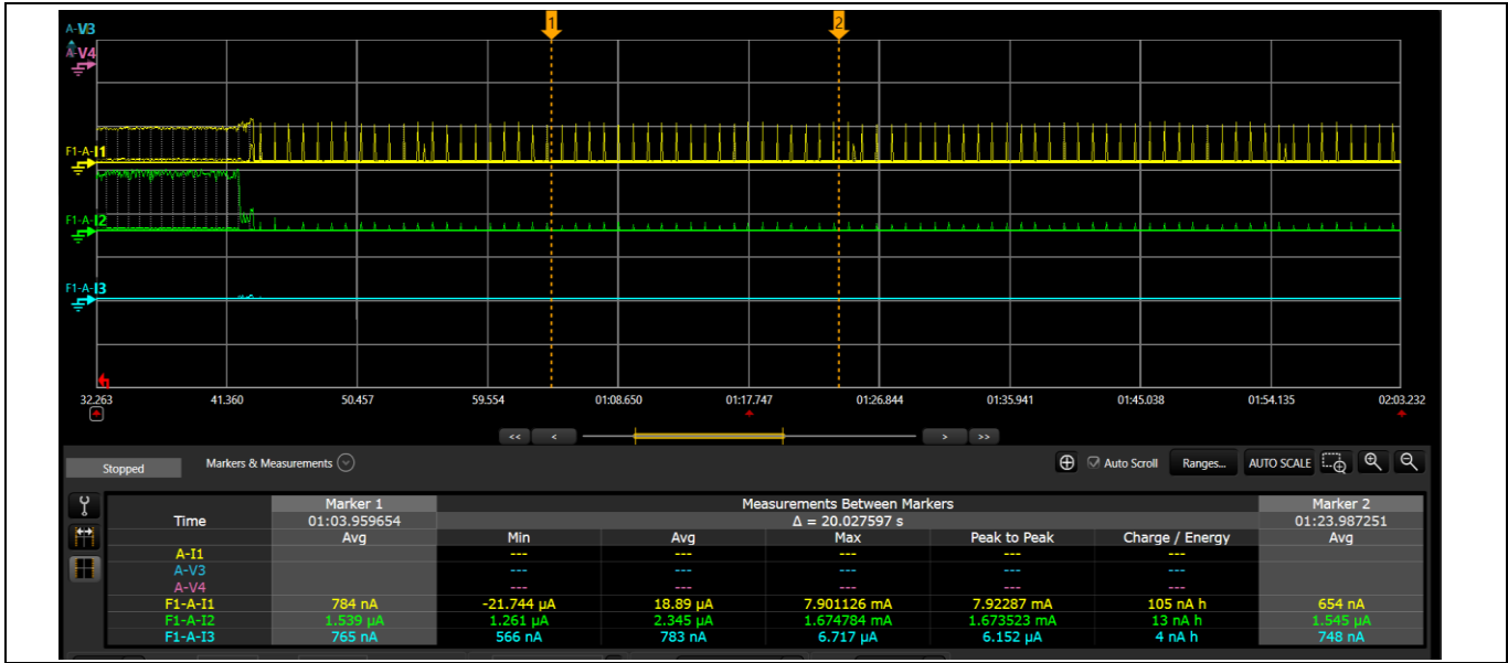
Figure 21 Deep Sleep connection idle with 1 s connection interval
