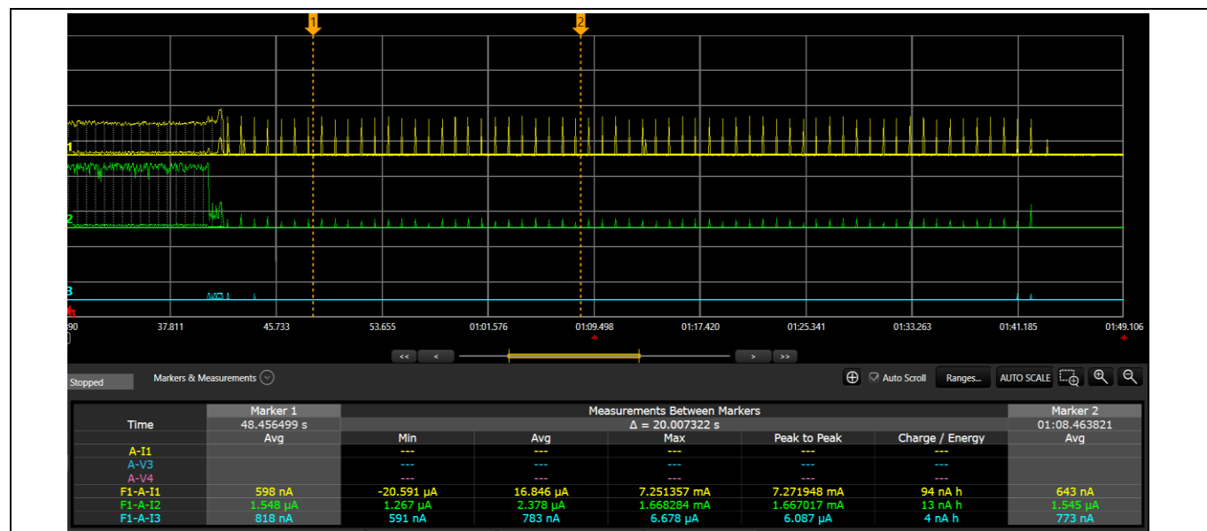
Figure 23 Deep Sleep RAM connection idle with 1 s connection interval
