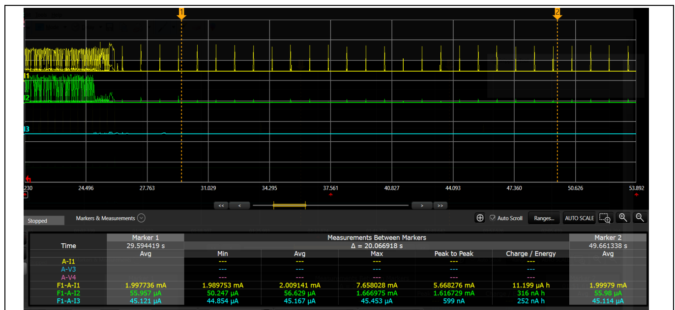
Figure 18 Sleep connection idle with 1 s connection interval
