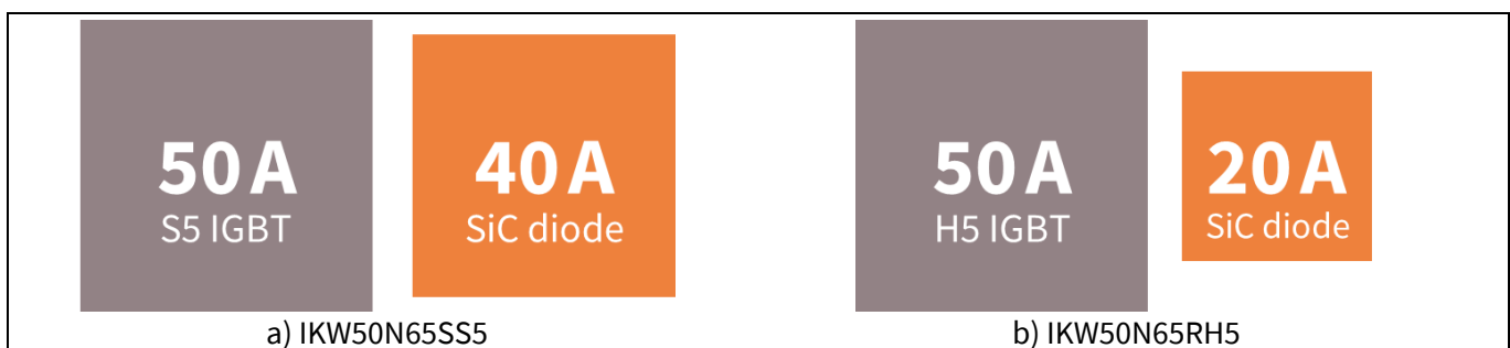
Figure 3 Diode current ratings using the example of two 50A devices: a) IKW50N65SS5 with full-rated diode, b) IKW50N65RH5 with half-rated diode.
