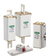
Extremely fast acting and offering high-speed performance up-to 1500 V dc, these fuses range from 80 A to 1400 A in the smallest IEC standard NH XL package sizes. Available with multiple mounting terminations including flush-end, DIN, and bolted blade style.
