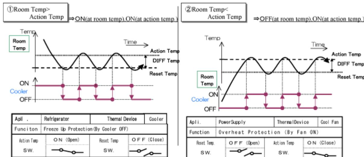
So let's say that you want to cut off current to a heating coil as soon as a specific temperature is reached or you want to enable a cooling fan when that temperature is reached. Sure you can do that with the typical clap-trapery of a thermistor connected to the A/D input of a microcontroller and then that controls a power FET or a relay (oh yeah, and software).
