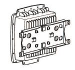
**Step 2:** Thread the two supplied metal mounting straps through the large slots on the mounting plate and then put the straps around the pole.
