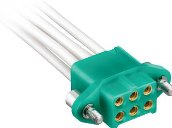
**M300 Series** – These low-profile 3mm pitch hi-rel power components feature a 4-finger contact design that maintains connection integrity regardless high levels of vibration and shock. The current rating is 10A per contact, with 3-contact single row, plus 6-contact and 10-contact double row arrangements available. A 1000 mating cycle durability is supported.
