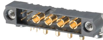
**Mix-Tek** – Harwin's Mix-Tek product offering combines power and signal connection, in order to save valuable space within densely-packed electronic designs, such as robotics. The power contacts are rated up to 40A, while the signal contacts have a 3A rating. The connectors can accommodate up to power contacts and up to 12 signal contacts, with a wide array of different options covered.
