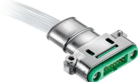
**Gecko-SL** – Compact and lightweight, but still also ultra-rugged, these 1.25mm pitch connectors are optimised for high-density electronic deployments where available space is limited. Their robust construction and stainless steel screw-lok mechanism protects them from elevated levels of shock (50g) and vibration (20g/2000Hz). Furthermore, a -65°C to +150°C temperature range is supported. Each of the beryllium copper plated contacts has the capacity to deliver 2A of current.
