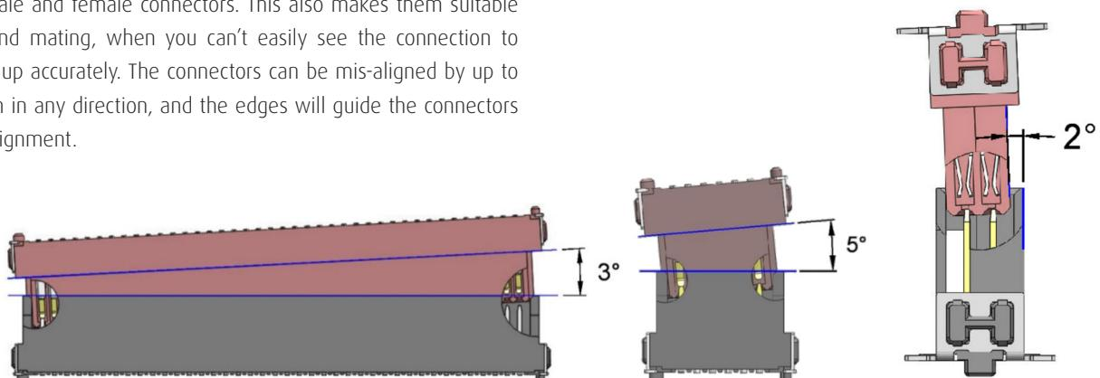
These considerations are very useful when modules are replaced or maintained in the field, especially if customers are allowed access to these connectors.
