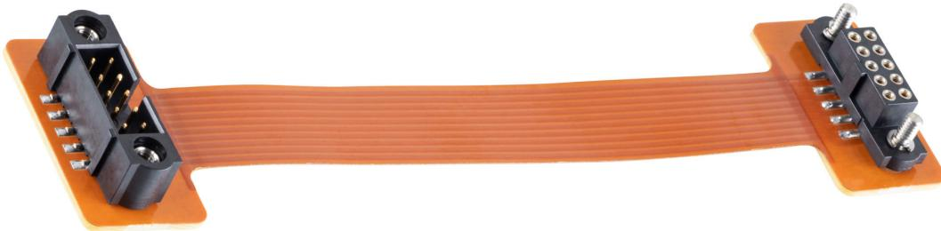
Connectors can be either SMT soldered or through-hole soldered, normally with shorter tails than intended for standard PCBs. This connection type has been common in high-density consumer electronics for many years (cell phones, laptops, flat-screen TVs), but the drive to minimize the size of electronics in all applications is making the use of FPC more widespread.
