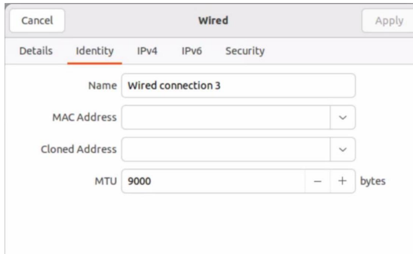
Figure 2-4 ConnectX connection identities/settings on each QSFP port
