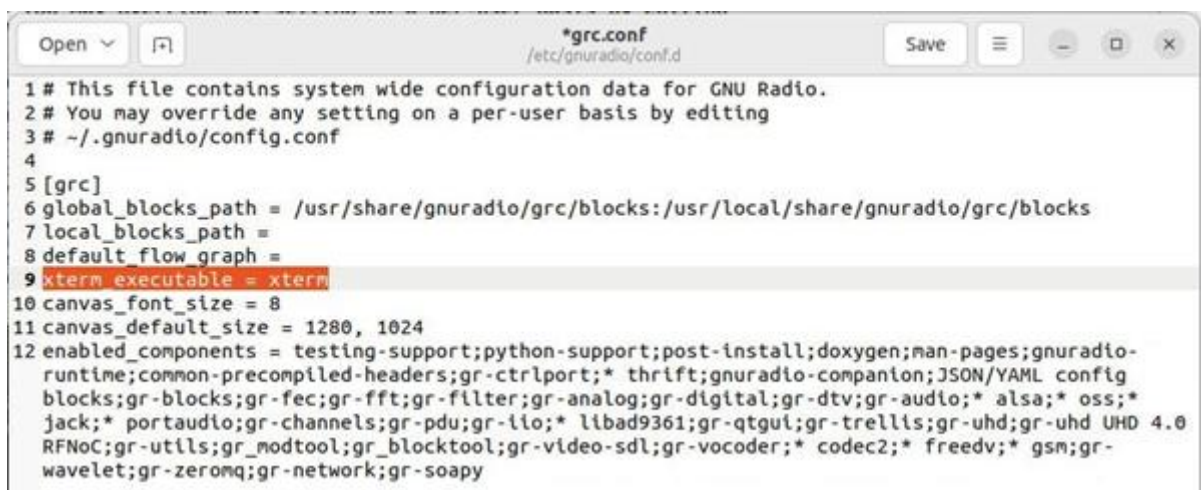
Figure 7-1 grc.conf modifications for GNURadio installation on L4T IGX BaseOS
