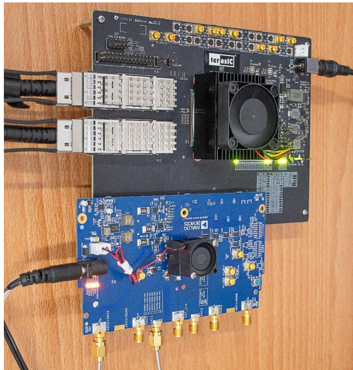
Figure 2-3 HSB100G and AD9986 connected and powered
