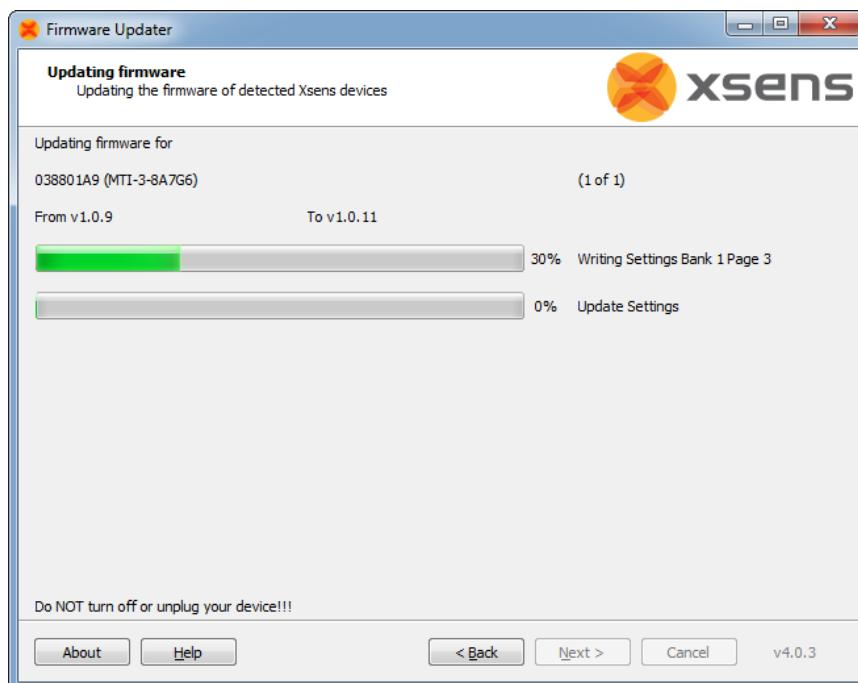
When the firmware update process is finished, the Firmware Updater provides a summary of the updated devices and firmware versions.
