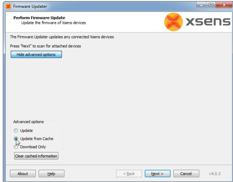
The Firmware Updater will check whether the firmware is available in cache. If the firmware is available, the following screen will be shown:
