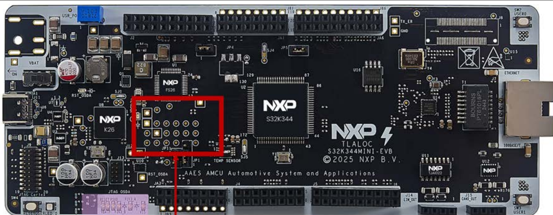
Power Test points/pads
