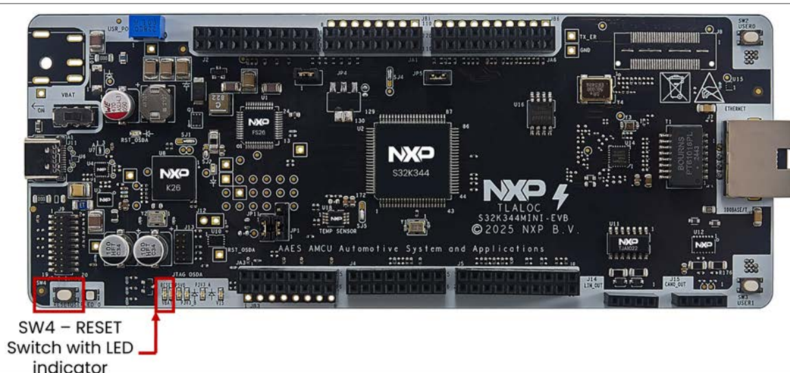
Figure 9. FRDM-A-S32K344 - JTAG connector and reset switch
