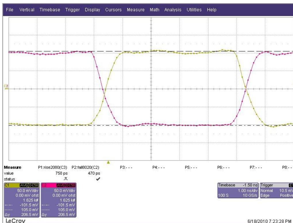
Figure 2.4. Typical Differential Output Waveform > 200 mV from Hardware Test
