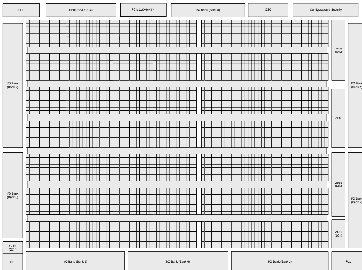
Figure 2.1. Simplified Block Diagram, LFCPNX-50 Device (Top Level)
