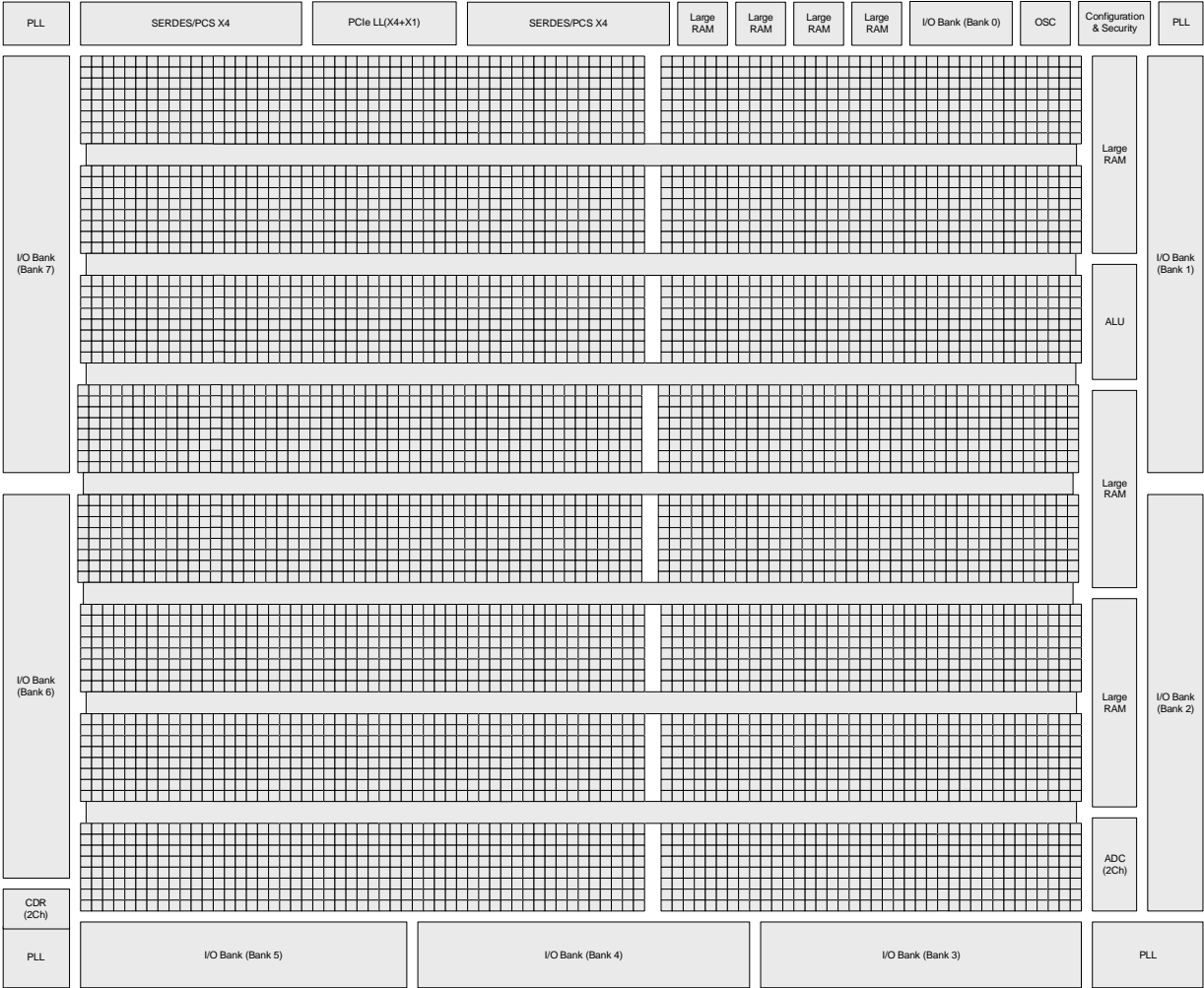
Figure 2.2. Simplified Block Diagram, LFCPNX-100 Device (Top Level)
