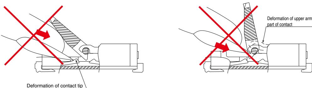
② As depicted below, the actuator was designed to rotate on a rotational axis. The actuator should be operated with this axis in mind.
