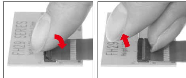
⑥ Do not pinch, lift or hook the actuator (as shown below), these actions can damage the connector. (Do not perform any operations other than the rotating operation described in Step ② above.)
