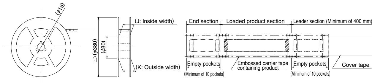
① The above dimensions are for the 5,000 piece reel. The outer diameter for the embossed 500 piece reel is φ 180mm.
