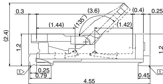
Note 1: The coplanarity of each terminal lead is within 0.1max.
