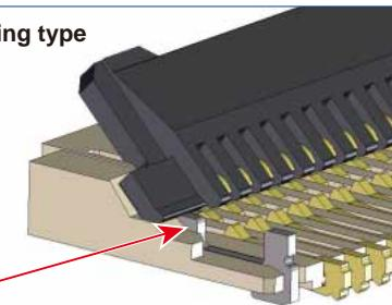
The reinforcing metal fittings support the actuator from below, this leads to an easier locking function.
