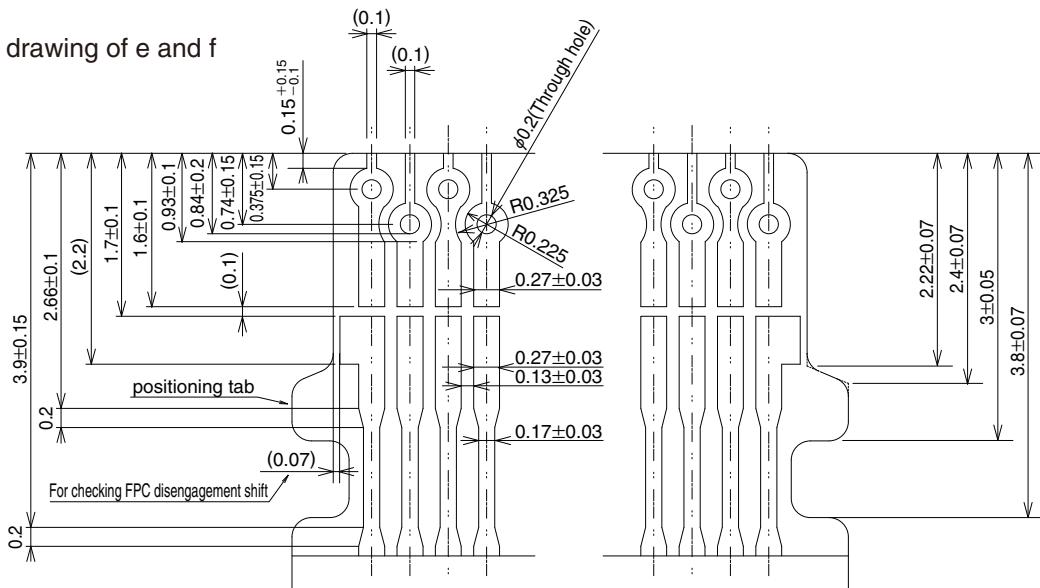
Note 1: To prevent pattern cutting, in case 4.7mm or more of stiffener cannot be secured, make the overlap amount to 0.5mm or more.
