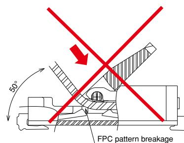
\*To avoid this problem, we recommend that consideration be given to insure the proper spacing needed to secure the FPC on the board. The length of the FPC should be considered as well because insertion becomes difficult with FPC that is too short.
