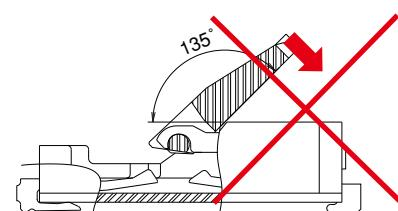
⑤ To close and lock the actuator after the FPC has been inserted; apply force on the center of the actuator to engage the lock. Applying pressure to the edges of the actuator might damage or deform the actuator.
