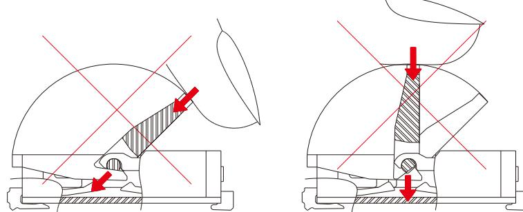
④ The actuator is designed to open to a maximum of 135 degrees, trying to open it farther than that will lead to damage or disengagement. The force applied should be less than 1 N. (Refer to the drawing below.)
