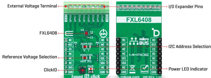
Expand 16 Click uses a standard 2-wire I2C interface to communicate with the host MCU, supporting clock frequency up to 400kHz. The I2C address can be selected over the ADDR SEL jumper. The FXL6408 has three reset options: power-on reset, over the software, and the RST pin by writing the logic LOW. When the event occurs, the I/O expander will assert the host MCU over the interrupt INT pin.
