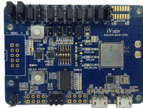
The development kit for EVIA USB comes with everything needed for verification of IEEE 802.11n/ac functionality on USB interface. The package contains the following contents:
