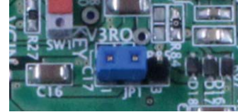
Figure 10. Jumper Switch JP1
