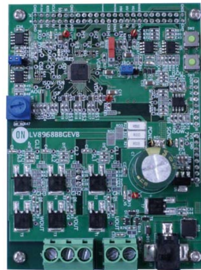
Figure 1. LV8968BB Evaluation Board
