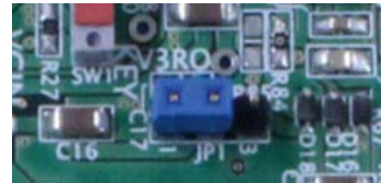
Figure 14. Jumper Switch JP1
