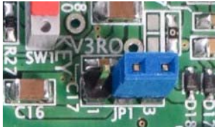
Figure 12. Jumper Switch JP1
