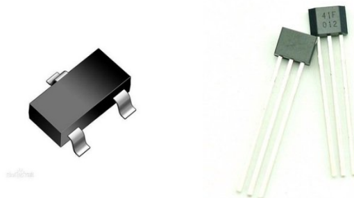
Figure 3: Hall IC (Outputs Logic Polarity Signal)
