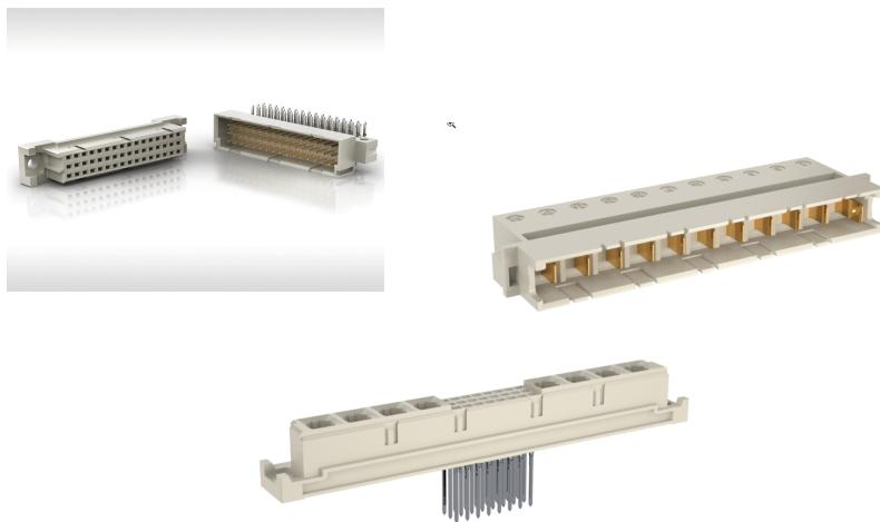
**ERNI's DIN 51612/IEC 60603-2 is available in both signal and power. Originally introduced in 1968, ERNI has continued to develop this powerful and proven signal solution has a pitch of 2.54 and the accompanying power module comes in at 5.08mm. ERNI offers DIN at the finished connector, cable assembly and sub-assembly levels. With more than 13 different shapes up to 160 contacts, the original DIN is diverse, robust, and flexible.**
