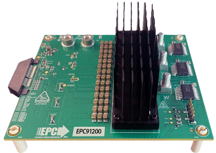
Figure 3: EPC91200 Evaluation board with heatsink attached
