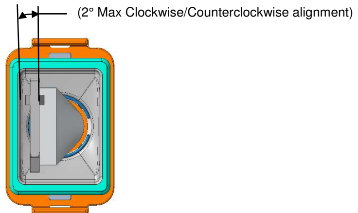
Figure 8c: HV Tab ultrasonic welding to ferrule alignment
