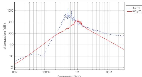
Typical Insertion Loss: Asym: 3L/N-GND, Sym:L-L
