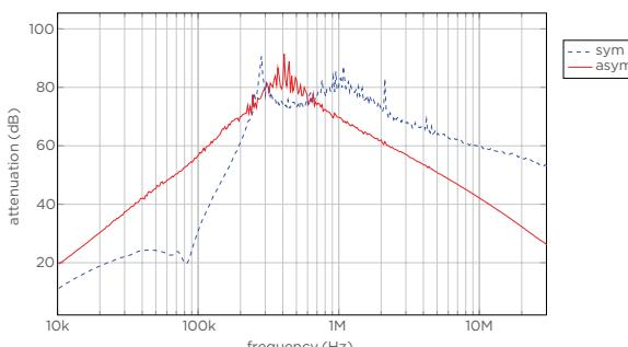
Typical Insertion Loss: Asym: 3L/N-GND, Sym:L-L
