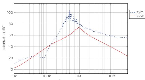
Typical Insertion Loss: Asym: 3L/N-GND, Sym:L-L
