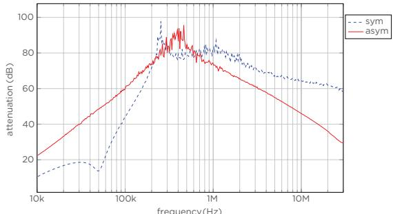
Typical Insertion Loss: Asym: 3L/N-GND, Sym:L-L
