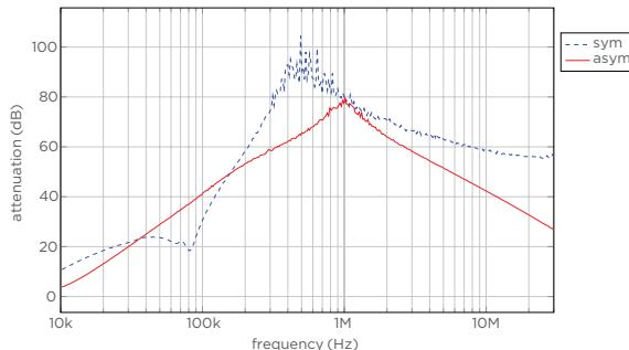
Typical Insertion Loss: Asym: 3L/N-GND, Sym:L-L
