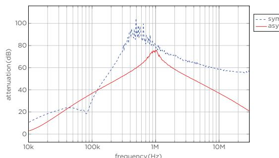
Typical Insertion Loss: Asym: 3L/N-GND, Sym:L-L
