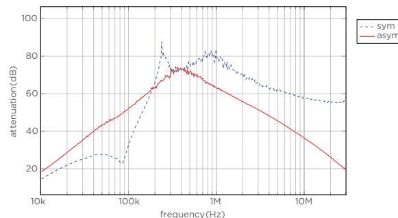
Typical Insertion Loss: Asym: 3L/N-GND, Sym:L-L
