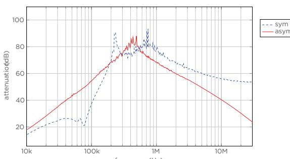
Typical Insertion Loss: Asym: 3L/N-GND, Sym:L-L
