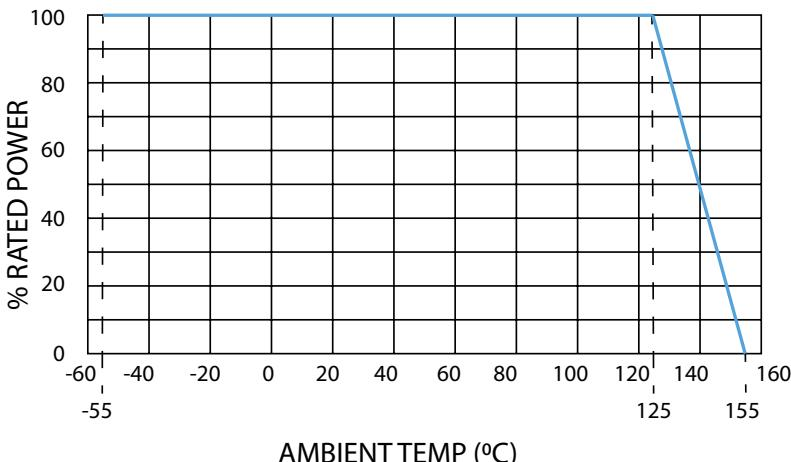
**Note:** When the terminal part temperature of the resistor exceeds the rated terminal part temperature shown above, the power shall be derated according to the derating curve.
