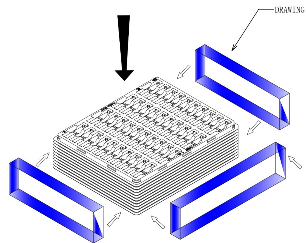
STEP 2: 10 TRAYS/STACK = 400 PCS, THE UPPER AND LOWER LAYERS CAN NOT BE MISALIGNED. FIX WITH PE FILM. (THE TOP TRAY IS EMPTY)
