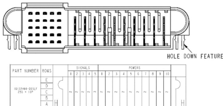
With respect to signals "3" in Columns 5, refers to the shortest level signal pin; the "shortest" pins are the "last to make, first to break" in the mating sequence
