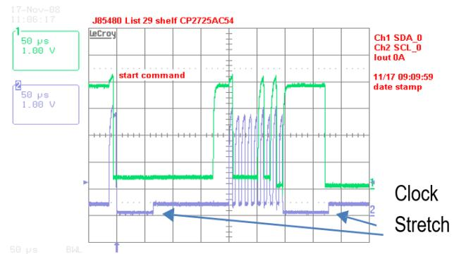
**I<sup>2</sup>C Bus Lock-Up detection:** The device will abort any transaction and drop off the bus if it detects the bus being held low for more than 35ms.
