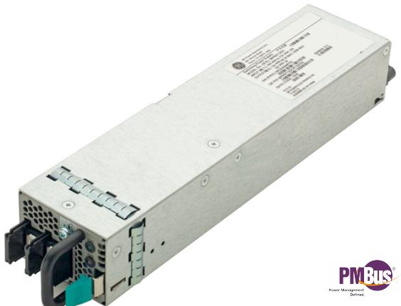
The MPR0712DC series provides high efficiency isolated power from the DC input mains. The industry standard PMBus® compliant I2C communications bus offers a full range of control and monitoring capabilities. The SMBAlert signal pin automatically alerts customers of any state change within the power supply.
