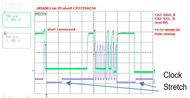
**I<sup>2</sup>C Bus Lock-Up detection:** The device will abort any transaction and drop off the bus if it detects the bus being held low for more than 35ms.
