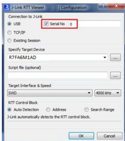
4. For parts other than Cortex-M33, click **OK**. For MCUs based on Cortex M33 Core, refer to the Appendix.
