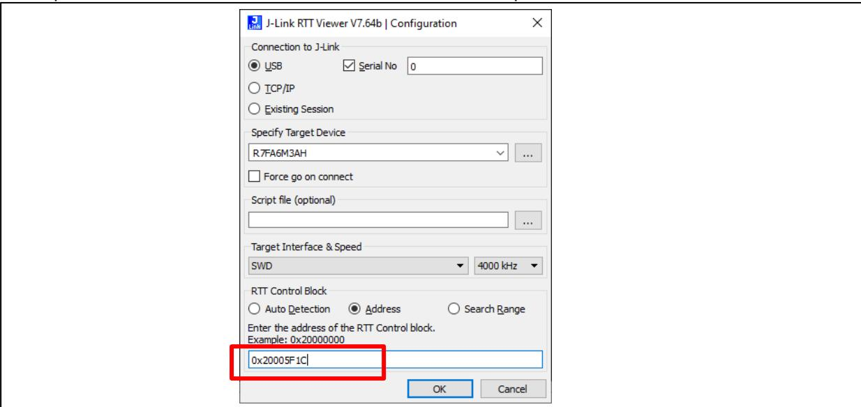
The image shows the 'J-Link RTT Viewer V7.64b | Configuration' dialog box. It has sections for 'Connection to J-Link' (USB selected), 'Specify Target Device' (R7FA6M3AH selected), 'Target Interface & Speed' (SWD selected, 4000 kHz), and 'RTT Control Block' (Address selected, address 0x20005f1c entered in the input field). The input field for the address is highlighted with a red box.
