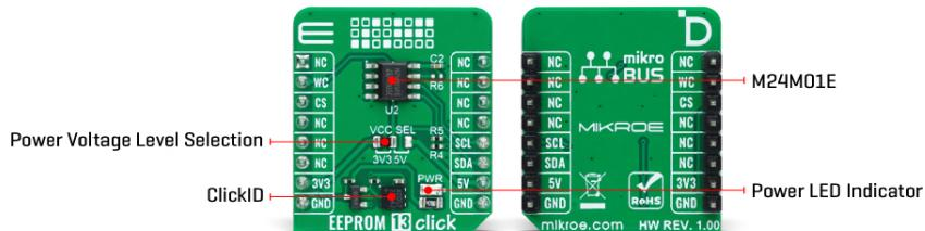
EEPROM 13 Click uses a standard 2-wire I<sub>2</sub>C interface to communicate with the host MCU, supporting standard, fast, and fast mode plus with up to 1MHz of frequency clock. The write control WC pin serves as a write protect option and is active with a High logic state.
