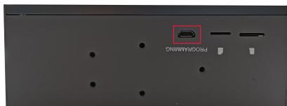
3. Connect the power cord and USB flashing cable (Micro-USB to USB-A).
