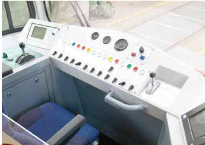
An HMI System for a locomotive could include alarm and status signals from a variety of the vehicle’s subsystems.
