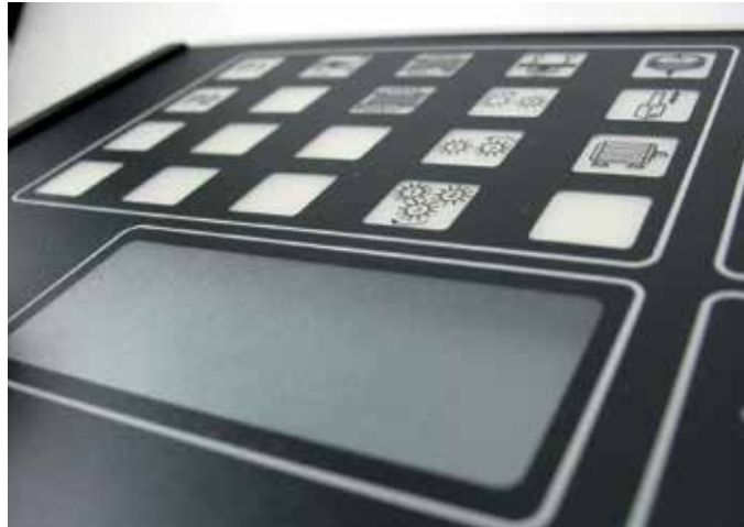
Short-travel technology can be provided with flush resilient surfaces.
