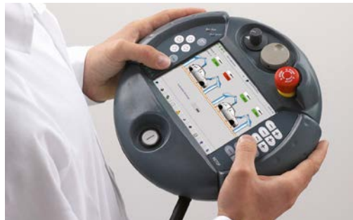
Handheld control unit with a display and electromechanical devices.
