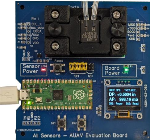
The Amphenol All Sensors AUAV Evaluation Kit is an essential tool for engineers and developers seeking to simplify the design, testing, and validation process of the AUAV sensors.
