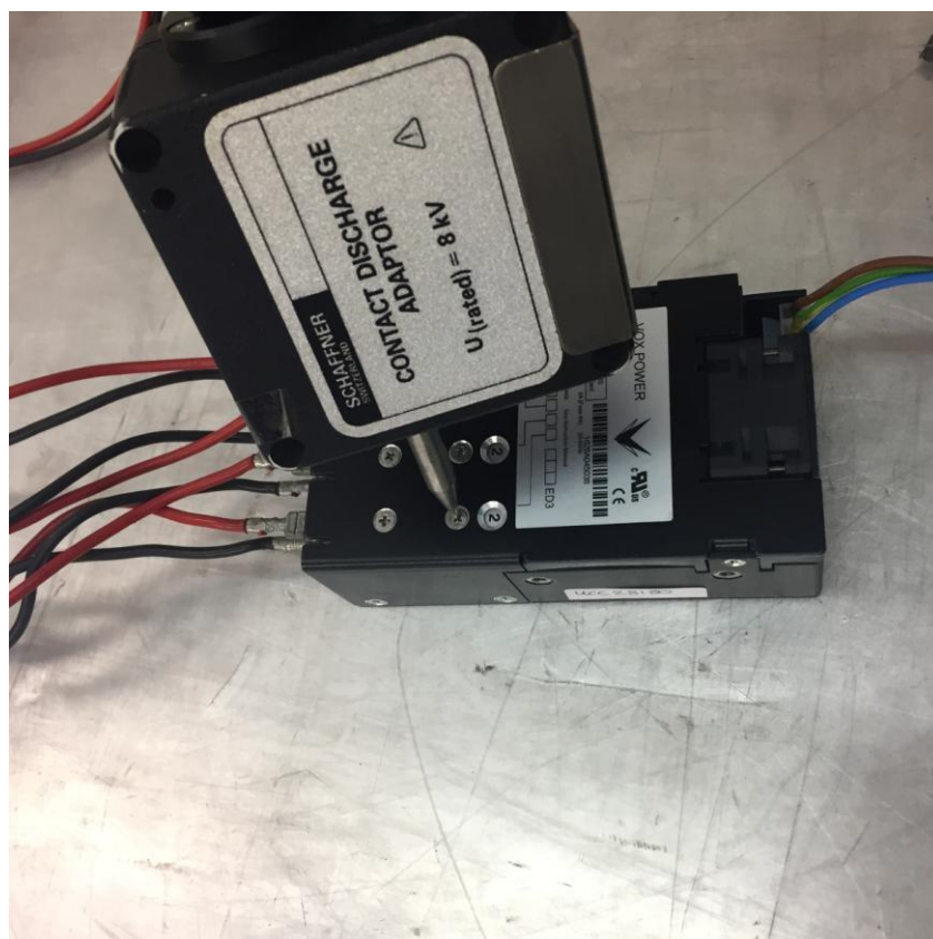
Figure 7: ESD Test Set up
