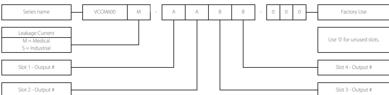
Industrial input module has ITE approvals (IEC62368 & IEC60950), Medical input module has medical approvals (IEC60601)
