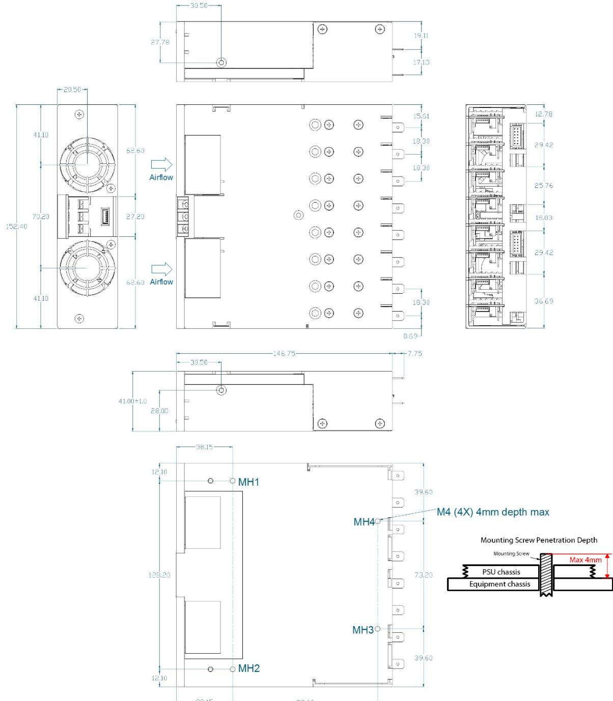
**TOLERANCES** unless otherwise stated - All dimensions in **mm** and according to DIN 2768-1/-2 CLASS C
