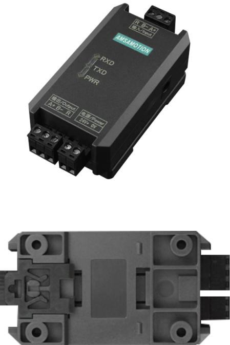
**Single Repeater:** For point-to-point, the repeater can connect with one 485 output device. The repeater can also extend the communication distance to 1200m. For point-to-multipoint, the repeater can connect thirty-two 485 output devices. The distance between the adjacent 485 devices cannot be more than 10 meters and the total length of the bus is extended to 1200 meters.
