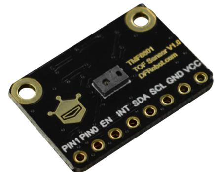
The TMF8801 sensor features a built-in histogram that delivers dynamic cover glass calibration and crosstalk compensation. The on-chip sunlight rejection filters help minimize the background light and noise. This sensor outputs data through a I<sup>2</sup>C fast-mode communications interface and an integrated microcontroller. Typical applications include 3D face recognition, proximity detection, presence detection, object detection, distance measurement, and collision avoidance.
