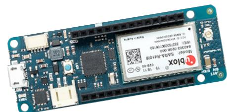
The Arduino MKR NB 1500 board offers a wide range of available interfaces, including I<sup>2</sup>S, I<sup>2</sup>C, UART, and SPI and operates at 3.3V. This board features ECC 508 crypto chip that effectively assures security in the communication process. Applications include field monitoring systems, intelligent parking, home and commercial intruder alarm, and fire alarm.
